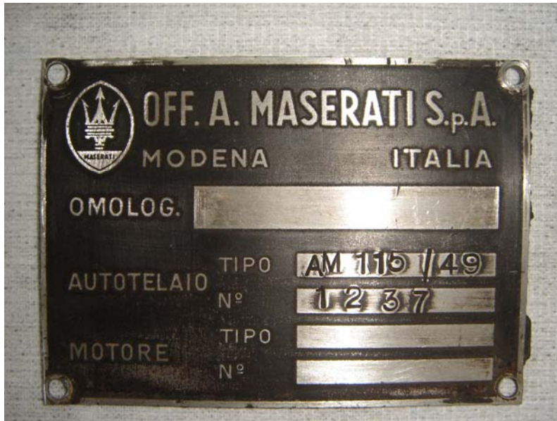
Pic. 7: Data plate from an original Ghibli SS Spyder
