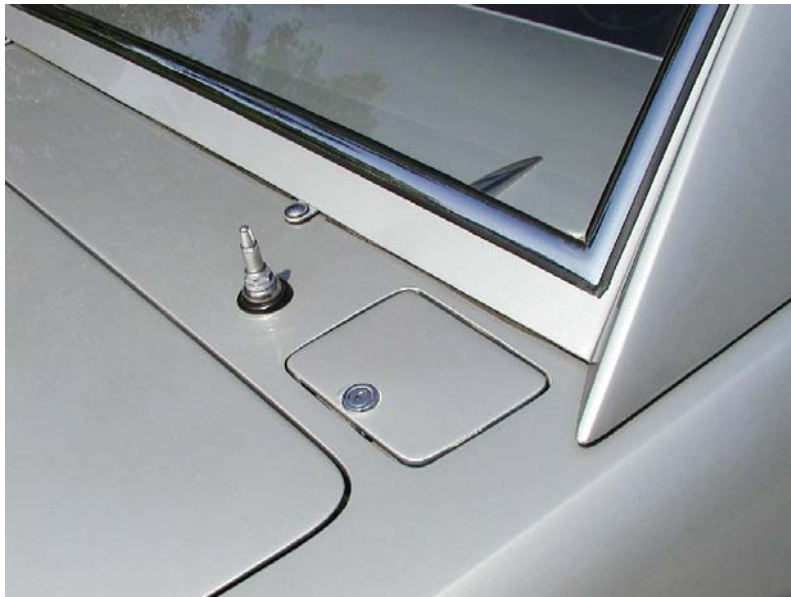
Pic. 112: Electric antenna is located next to the right fuel tank filler. Note hard top mounting bolts.
