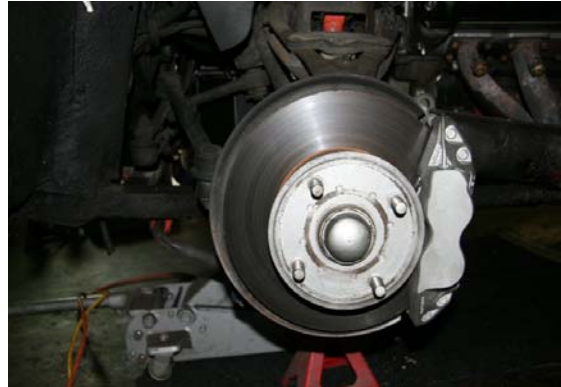
Pic.22: More common single front disc caliper
