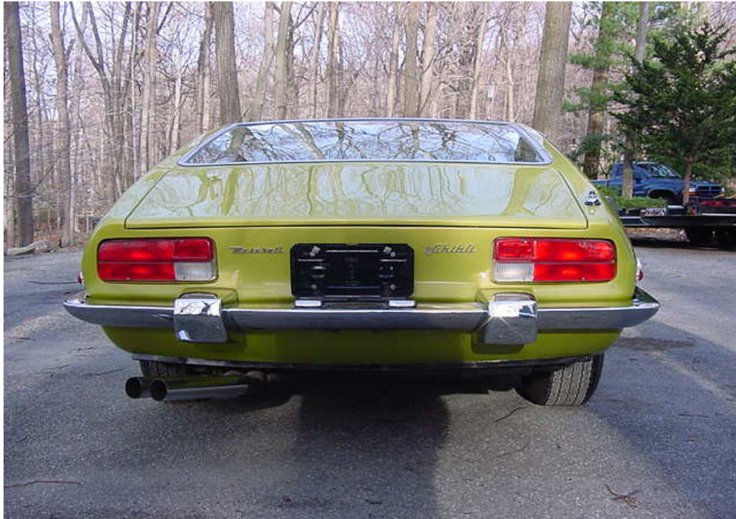
Pic.43: Rear chrome over-riders as found on most late USA cars. Note position to taillights.
