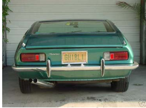
Pic.41&42: Rear chrome over-riders with inset rubber. Note the off-set position to the taillights.
