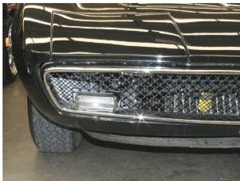
Pic.52&53: Early European style front white turn signal lights, mounted low on grille surround.
