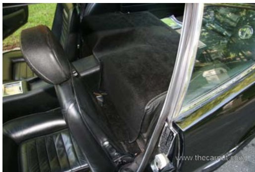
Pic. 91&92: Many cars had the cushions covered with the carpet extending from the boot to the lower rear part of the front seats.
