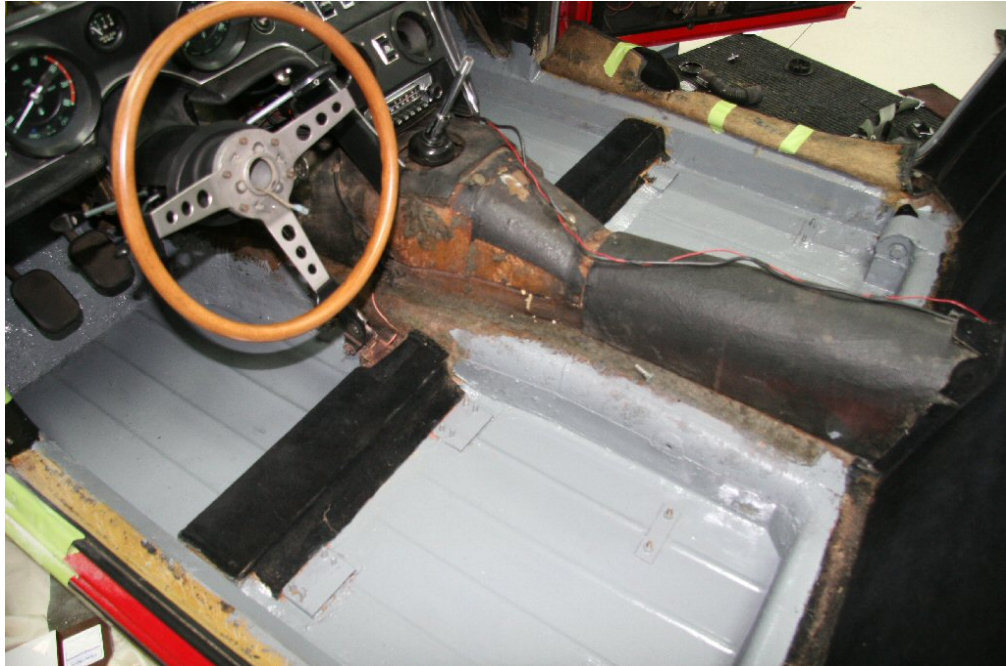
Pic. 105: Double floor on a Ghibli Sypher.
