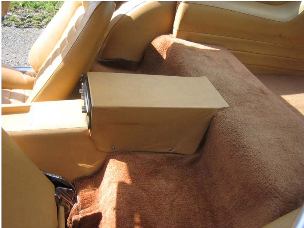
Pic.123: Radio/cassette, dealer mounted under a box on the rear deck (without carpet cover).
