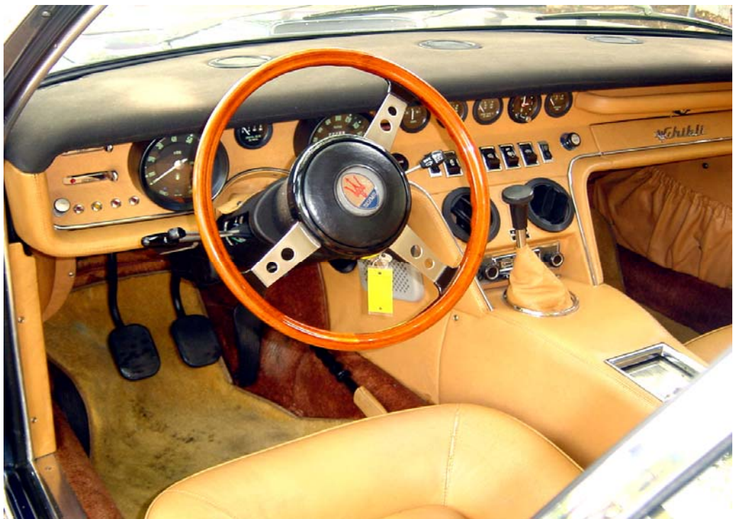
Pic.81: USA steering wheel with horn button with Maserati logo from a late 1972 Ghibli.
