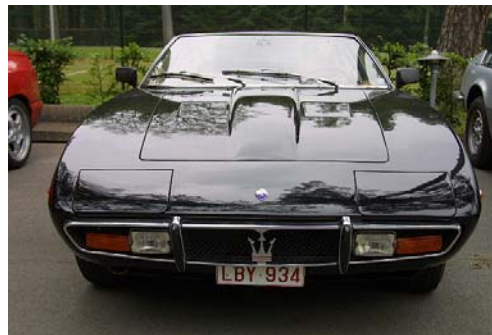
Pic.56&57: Late style front turn signal lights, two-colored (Europe) and amber only (US). Note fog lamps mounted outside of the grille.
