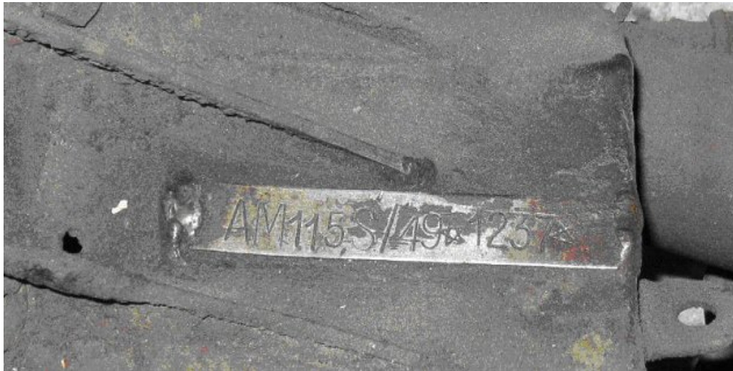
Pic. 8: Original chassis plate; notice the stars before and after the serial number. The "S" was used in this situation.
