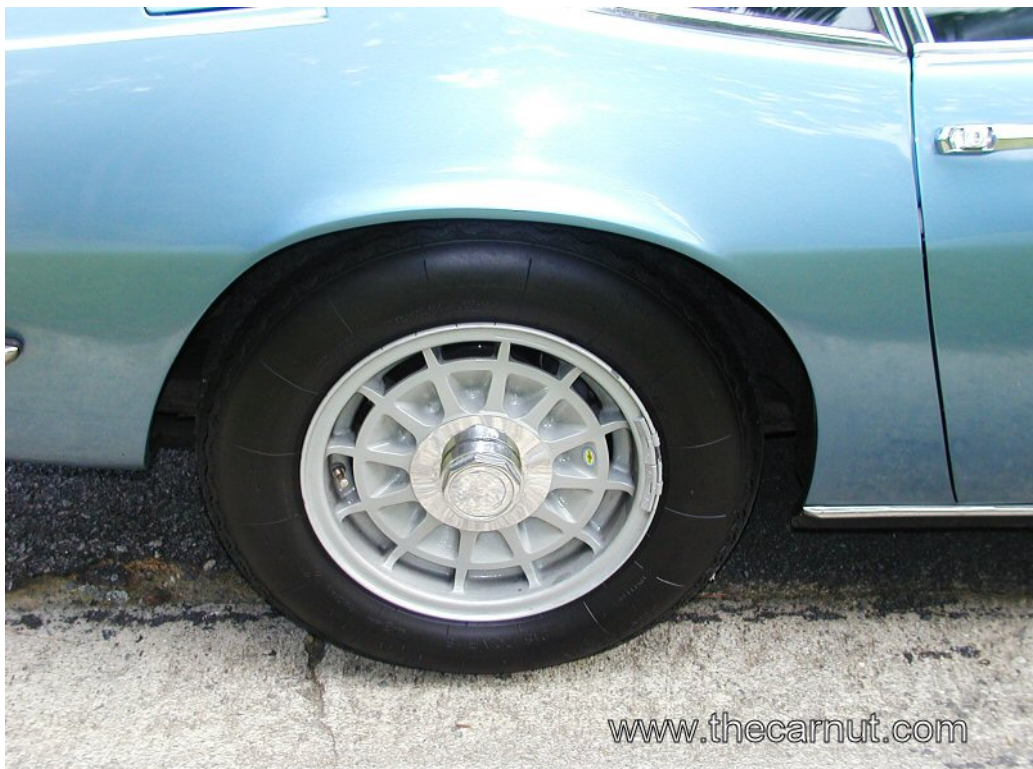
Pic.34: Campagnolo starburst wheel: Similar appearance to the early knock-offs, but it's actually a bolt-on wheel with an attractive center cap that hides the bolts.
