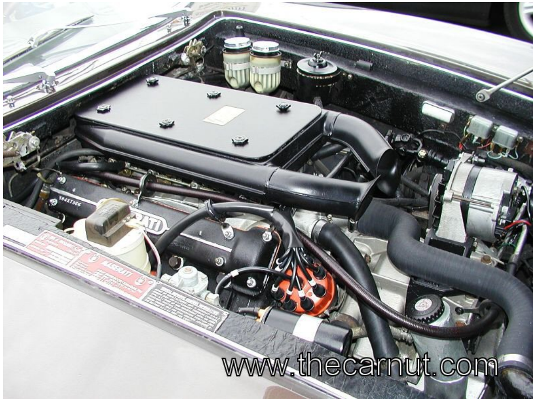
Pic.18: Most 4.9 liter engines destined to the USA came with a rectangular air box. The Euro versions mostly had the oval air box and are visually undistinguishable from the 4.7 version.
