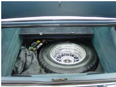
Pic.99&100: The trunk had a one piece top-deck covered by carpet.
