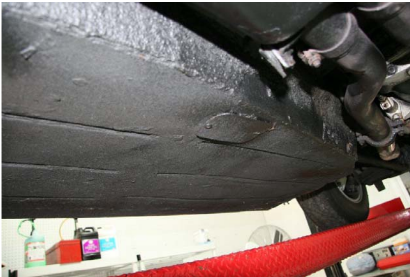
Pic.110: Access panel for hand brake cable on a Spyder.
