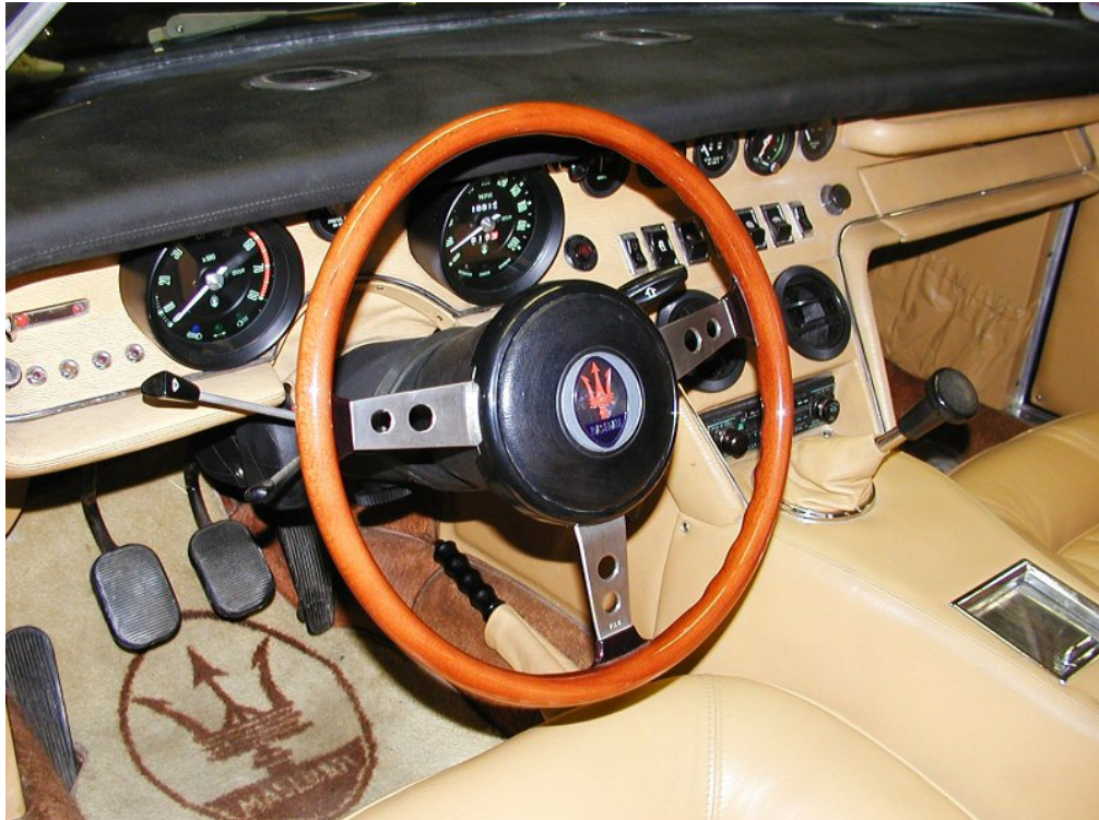
Pic.75: Vitaloni stalk on a USA steering wheel with the large horn button and logo. The stalk is fragile and expensive to replace.
