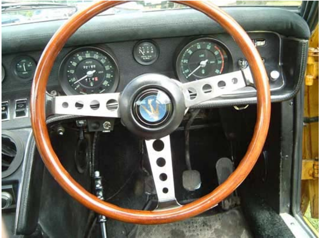
Pic.76: Wooden steering wheel with small horn button with black rim on this RHD Ghibli.
