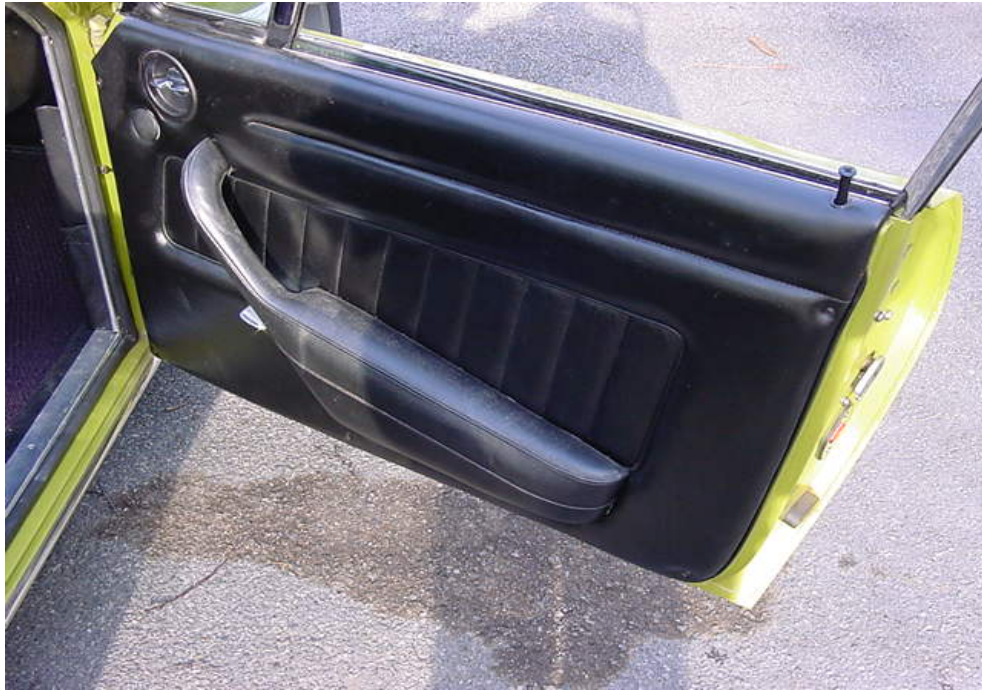
Pic.87: Mid-series style of door panel, here seen on a 1970 car.
