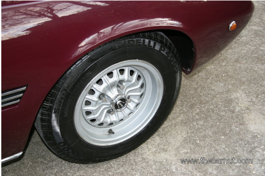
Pic.35: Another bolt-on wheel. This one looks like the style used on the Indy, but is 15'.
