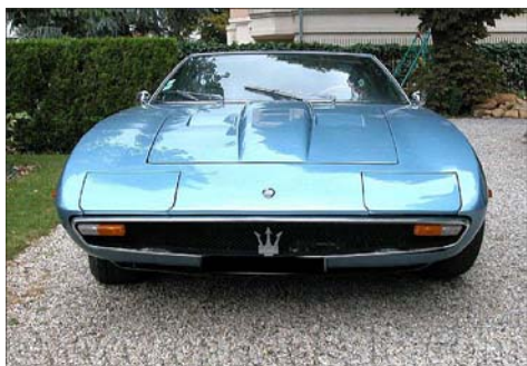
Pic.56&57: Late style front turn signal lights, two-colored (Europe) and amber only (US). Note fog lamps mounted outside of the grille.
