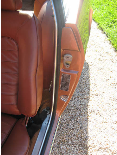
Pic.108&109: Trunk release levers on a coupé and a Spyder respectively, both US-cars with plate mounted on door post.
