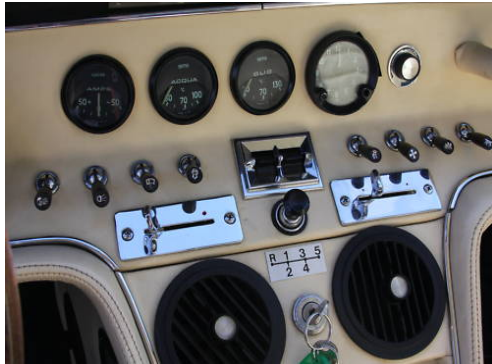
Pic.95&96: Hand-shifted US cars often had a small plaque (black, red or metal) mounted to the console indicating the shifting-scheme (see also Pic.101, 103).
