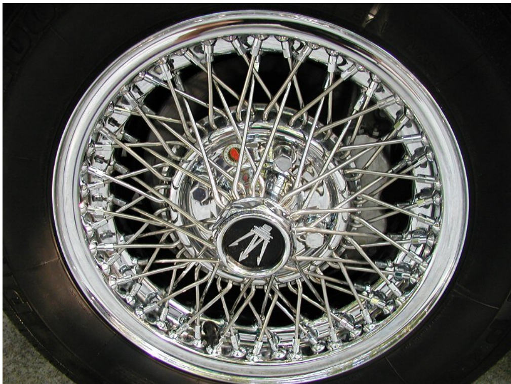
Pic.36: Borrani bolt-on wire wheel. On most Borrani wires the rim is alloy but on this wheel both the rim and center are steel.
