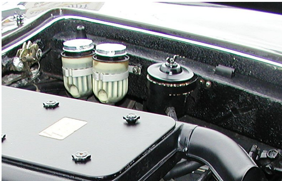
Pic.20: Easiest way to determine if the car has power steering is to look for the round black reservoir located next to the brake fluid canisters.
