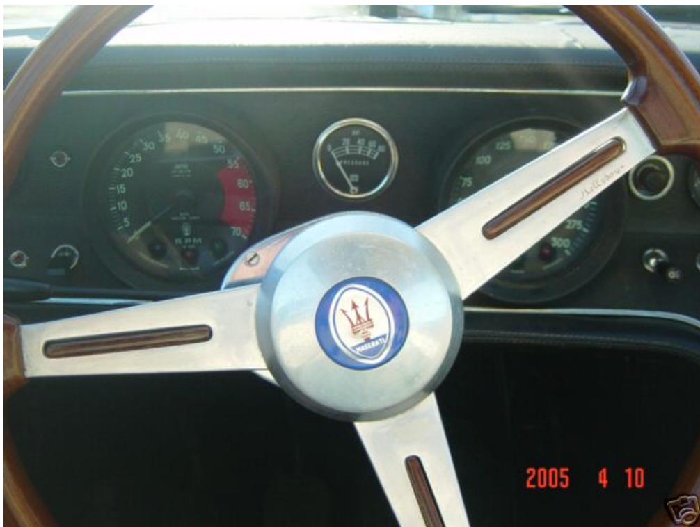
Pic. 79: The Hellebore wooden wheel on an early Ghibli (as found in late Quattroporte I).
