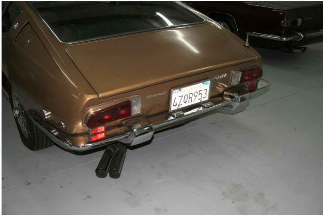
Pic.29: Dual exhaust to the side: common for USA cars.
