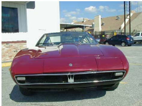
Pic.54&55: Early European style front white turn signal lights, mounted high and low on grille surround. Note fog lamps mounted behind the grille.
