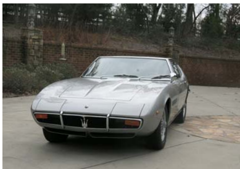
Pic.39&40: Front chrome over-rider, without and with inset rubber.
