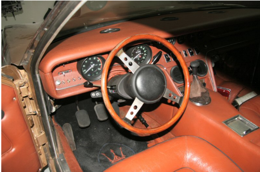
Pic.80: USA steering wheel with horn button without logo from a 1970 Ghibli.
