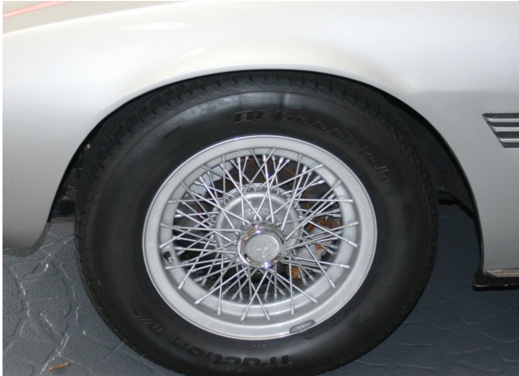
Pic.33: Knock-off Borrani wire wheel on an early car. Note the octagonal center spinner.
