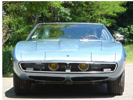
Pic.54&55: Early European style front white turn signal lights, mounted high and low on grille surround. Note fog lamps mounted behind the grille.
