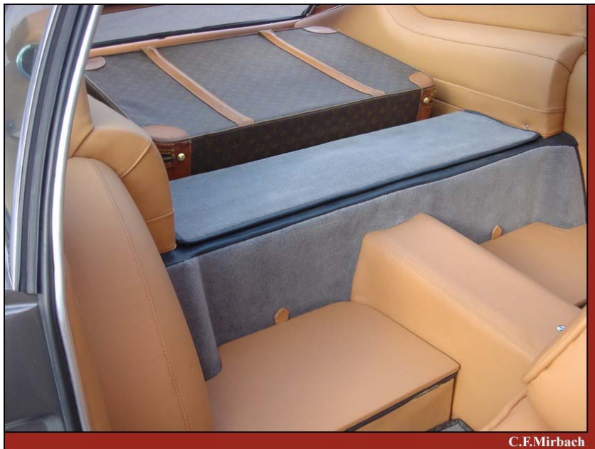
Pic.89: The rear deck had a compartment to be opened from the rear on each side.
