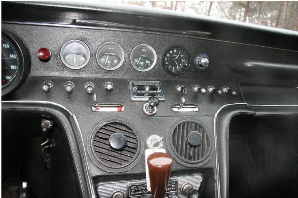
Pic.71: Toggle switches on a very early 1967.
