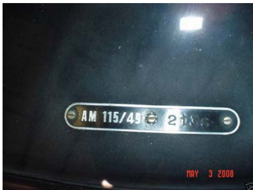
Pic.9&10: Later US cars had the AM-number screwed on a little plate to the dash-top on the driver's side. The dash plate can be easily seen through the windshield glass
