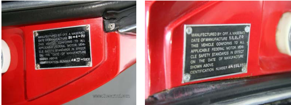
Pic. 11&12: US car plate with both the VIN and the date of manufacture on the left door pillar.
