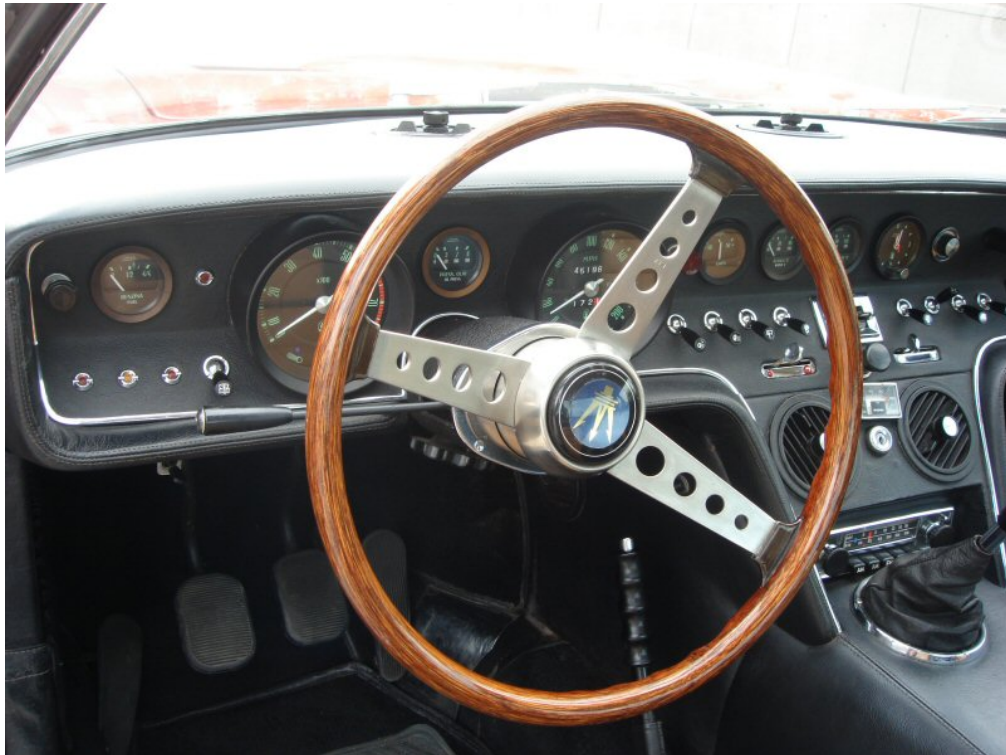
Pic.74: Lucas single stalk: Simple and reliable. Note early Euro (and early USA) steering wheel with small horn button without black rim.
