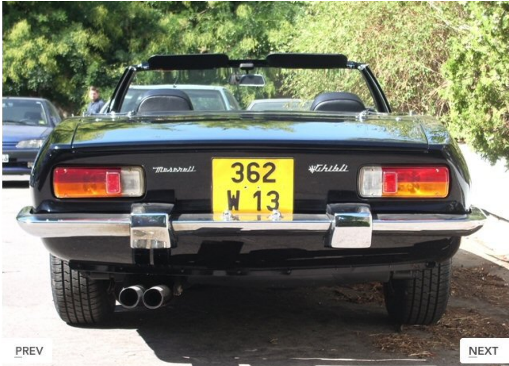
Pic.30: Dual exhaust straight back on this Euro Spyder.
