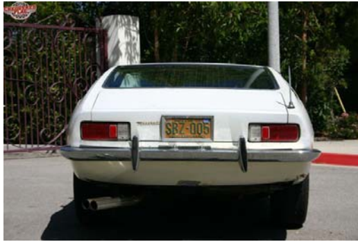
Pic.41&42: Rear chrome over-riders with inset rubber. Note the off-set position to the taillights.
