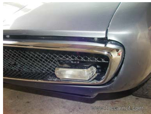
Pic.52&53: Early European style front white turn signal lights, mounted low on grille surround.
