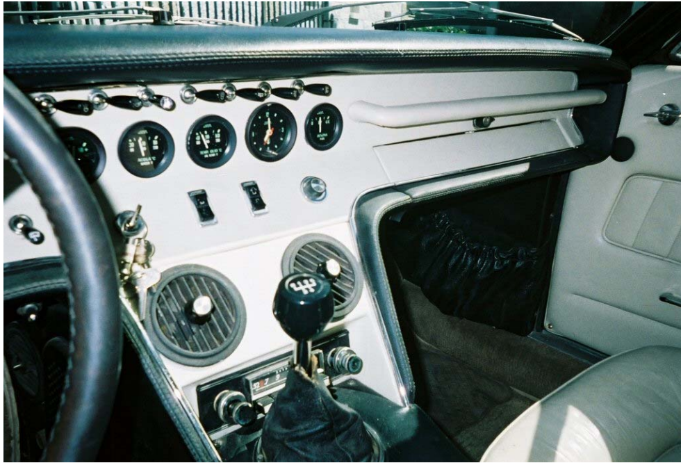
Pic.72: Interim toggle switch layout where the switches were placed along the top.
