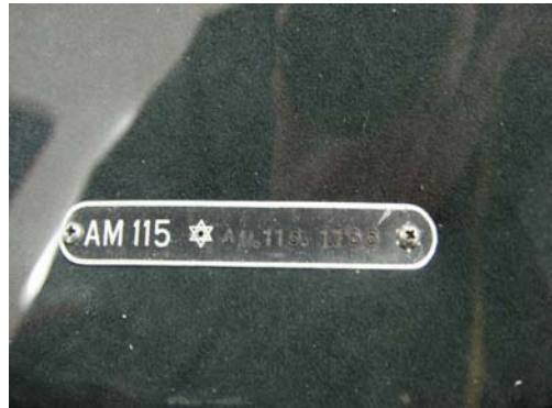
Pic.9&10: Later US cars had the AM-number screwed on a little plate to the dash-top on the driver's side. The dash plate can be easily seen through the windshield glass
