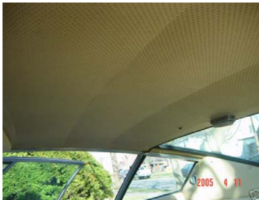
Pic. 106&107: On a coupé the interior light is mounted on the roof; on the Spyders they are mounted on the driver and passenger foot wells.
