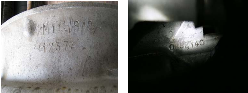
Pic. 13&14: Engine numbers from Spyder #1237 and from a 4.7 liter Spyder
