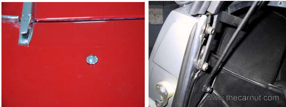
Pic. 118&119: Ghibli Spyder hard top mounting bolt. Some hard tops also had two side attachment bolts, but not all.
