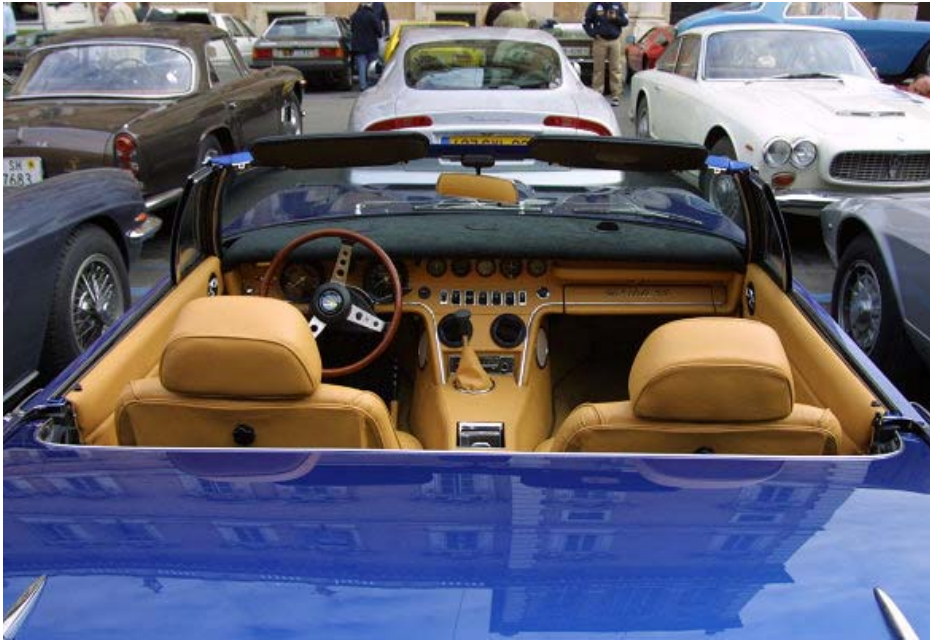
Pic. 113: Spyder sun visors are black and supported by black hinges; they are very similar to those found in Alfa spyders. Some restorers do them in the interior color.
