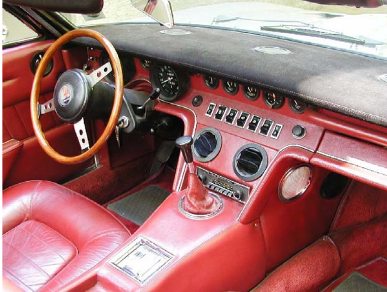
Pic.111: Loudspeakers mounted on either side of console on a Spyder. Note rocker switches and gear-shifter knob.
